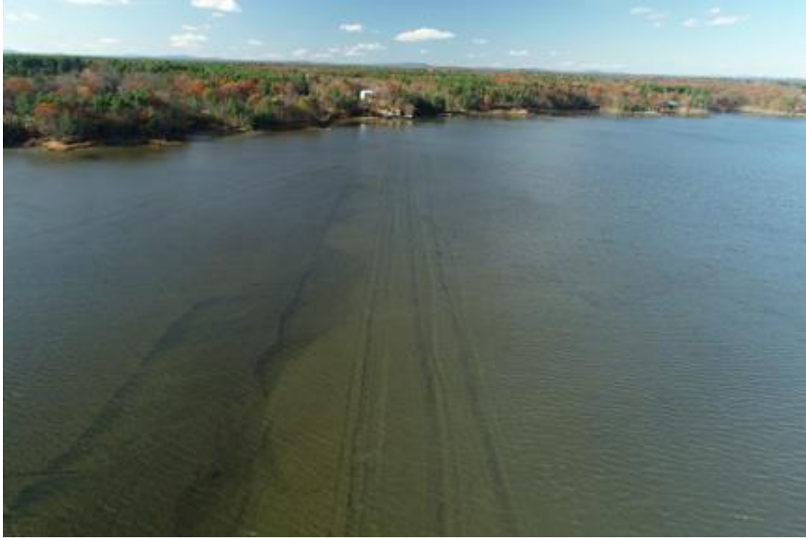
Photo 21. Cable 3, Flight 12, 11/06/2019. Jet plow tracks for the three cables are on the right. The dark tracks on the left are from the jet plow trial and a pre-lay grapnel run.
