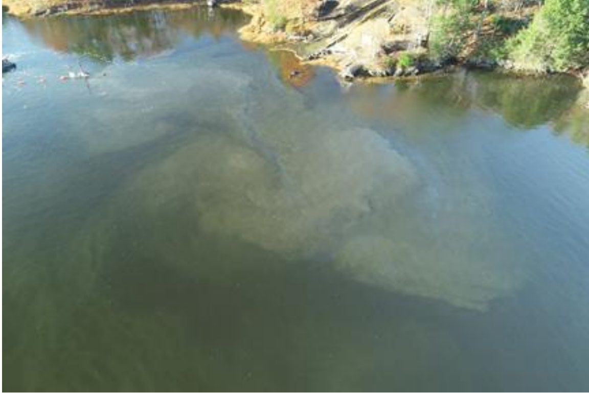
Photo 11. Cable 3, Flight 1, 11/06/2019. Approximately fifteen minutes after jet plow start on western tidal flats.
