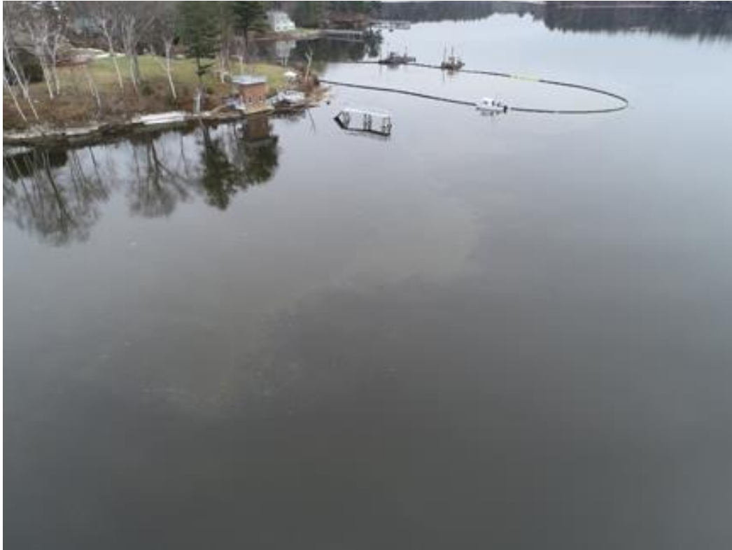
Photo 51. Hand Jet, Flight 8, 12/13/2019. Visible turbidity plume during ebb tide spill; no exceedances measured at mixing zone boundary.
